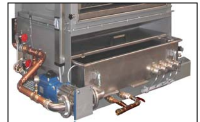
The filter washing system is situated between the two filter levels and has a movable manifold with washing nozzles. The water tank with circulation pump is underneath of the filter
